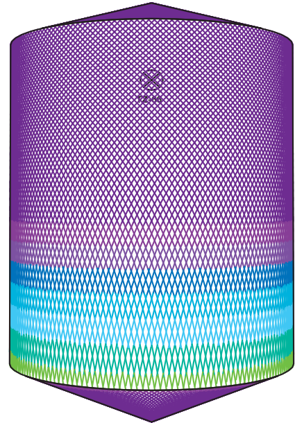
D8m H10m, Toftejorg TZ-66, 4 x \varnothing 10 mm, 0% Aika = 23.3 min, vedenkulutus = 10868 l
