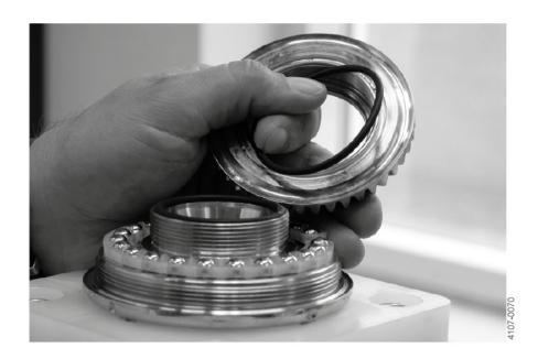
5. Carefully lift the hub nut (Pos. 15) of the nozzle head (Pos. 18) while keeping it horizontal to avoid damaging the surfaces.
