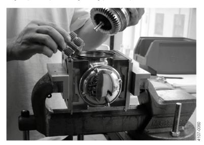
8. Remove the 3 screws (Pos. 13.5) securing the gear ring (Pos. 13.2) to the body using the torque wrench and NV8 socket long (TE81B156 + TE81B157)
