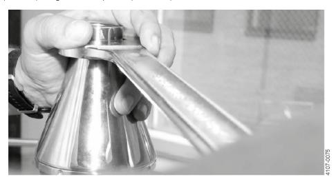
4. Loosen the cone (Pos. 1.1) by hand while lifting the cone vertically and finally remove the cone (Pos. 1.1)
