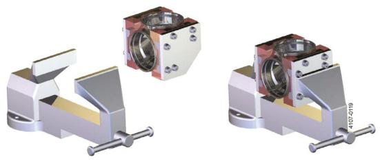
2. Mount assembled gear ring in body (Pos. 13.1). Tighten screws (Pos. 13.5) using the torque wrench (TE81B156+TE81B157) to maximum 5 Nm. Too much torque breaks the screws.
