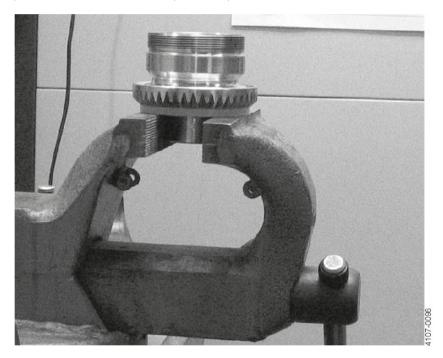
3. Place the ball retainer with balls (Pos. 5) onto the ball race on the stem (Pos. 8).
