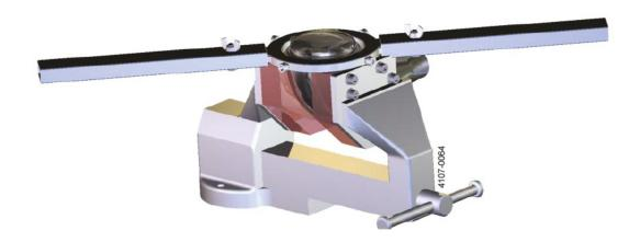
13. Remove hub nut (Pos. 15) from body. Lift vertically.
