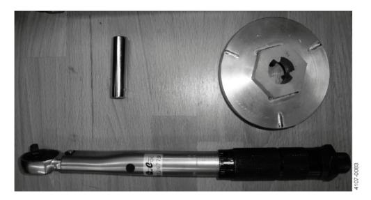
1. Mount the impeller turbine fixture (TE20J392) in bench vise. Loosen the shaft end (Pos. 3.4) using the torque wrench and NV9 socket long (TE81B156 + TE81B158) and unscrew with hand.
