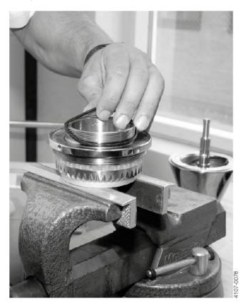
7. Carefully lift the stem nut (Pos. 4) of the stem (Pos. 8) while keeping it horizontally to avoid scratching the surfaces
