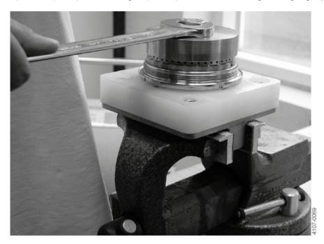
4. Remove the bevel gear (Pos. 14), the O-rings (Pos. 16 and 17) and the ball race (Pos. 5 – identical with the one used around the stem)
