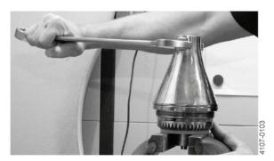
11. Check that the turbine assembly can move freely in the top part assembly
