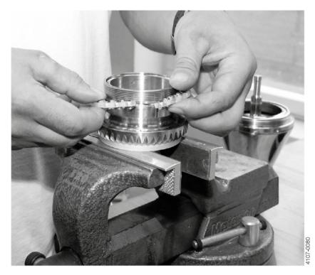
9. Extract gasket (Pos. 2) from the inside of the top of the cone (Pos. 1.1)
