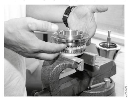
8. Remove the ball race (Pos. 5) from the stem (Pos. 8).
