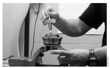
9. Carefully screw the cone (Pos. 1.1) onto the stem (Pos. 8) by hand.
