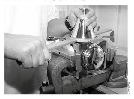
5. Loosen the stem nut (Pos. 4) by hand while lifting the cone (Pos. 1.1).
