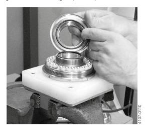
10. Screw the bevel gear (Pos. 14) on to the nozzle head (Pos. 18) thread by hand
