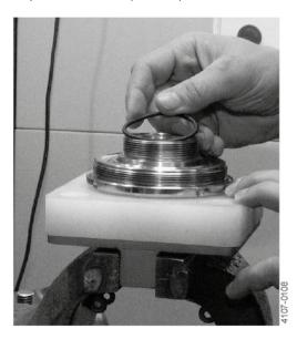
6. Preparation before mounting the bevel gear (Pos. 14) on nozzle head (Pos. 18): It is recommended to grease the nozzle head thread with food graded/FDA compliant grease. The grease reduces the risk of galling in threads. The grease is enclosed between the O-rings and, therefore, it will not come into contact with the cleaning media.
