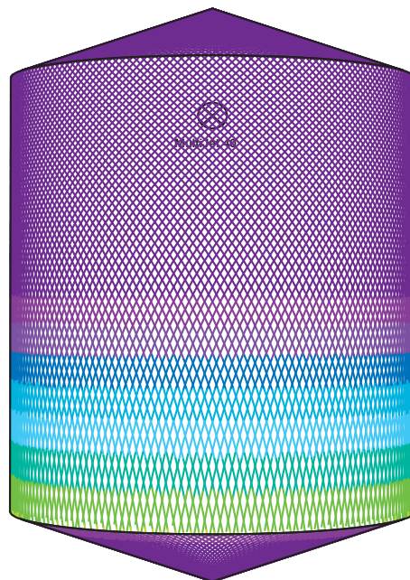
D5m H6m, Toftejorg MultiJet 40, 4 x \varnothing 6 mm, 100% Tempo = 18.2 min., consumo acqua = 3760 l
