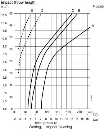
A. = 6.4 mm (1/4in)B. = 7.9 mm (5/16 in)C. = 9.5 mm (3/8 in)D. = 6.4 mm (1/4 in)E. = 7.9 mm (5/16 in) It is important to observe the technical data during installation, operation and maintenance. Inform personnel about the technical data.
