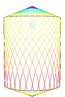
D21.3m (840"), H34m (1,340"), 2xØ11.11mm (2xØ7/16") Time = 6 min.
