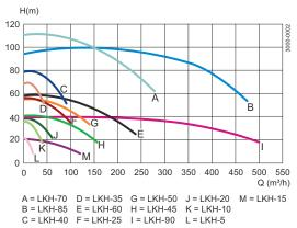
Frequency: 50 Hz Speed (synchr): 3000 rpm
