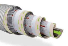
Flow pattern in a spiral-wound membrane element. Red is feed/retentate; yellow is permeate. The unique design of Alfa Laval spiral-wound membrane elements ensures the feed stream passes through the element under the best possible flow conditions. This secures the most efficient separation, superior flux, extended service life, and ease of cleaning.
