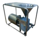
The dimensions of the Hybrid Powder Mixer are H 750 mm x W 826 mm x D 1340 mm. The weight of the complete unit is approximately 280 kg, mounted on wheels for easy handling. The motor is equipped with a VSD (18.5 kW) as standard. The maximum flow generated is  $26 \, \mathrm{m}^3 / \mathrm{h}$ . Maximum powder capacity is approximately 3000 kg/h, and the funnel powder volume is 50 l. Media wetted steel parts are in SS 316L (1.4404) and Duplex steel. Funnel, table and frame are in SS 304 (1.4301).
