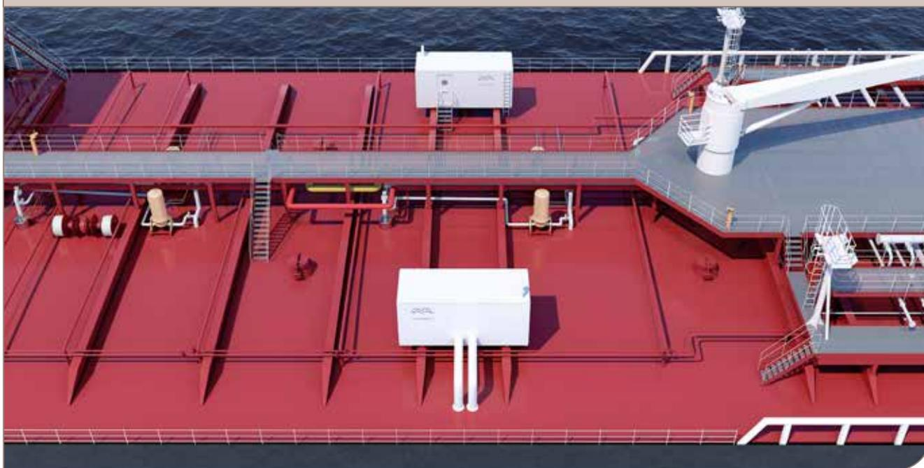
The technical teams for Alfa Laval ballast water treatment systems and Framo pumping systems have developed a solution for providing additional pumping head when PureBallast 3 Ex is installed in a deckhouse. By ensuring that the PureBallast 3 Ex system can handle its own pressure requirements, the optional booster pump unit (BPU) removes the need for changes in the existing ballast pumping system, thereby retaining its optimization and the vessel's cargo offloading rates.
