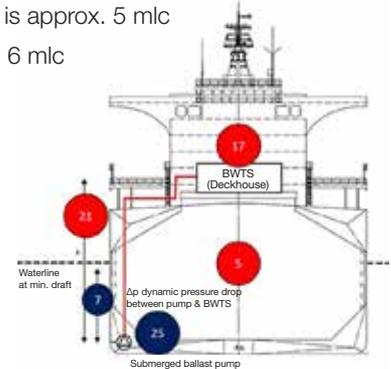
Since the ballast water treatment system requires around 17 mlc, the installed ballast pumps alone will not support proper backflushing, which may result in failure and the shutdown of cargo operations. Installing a BPU in the deckhouse will remove this problem by ensuring adequate discharge head in the ballast water treatment system.
