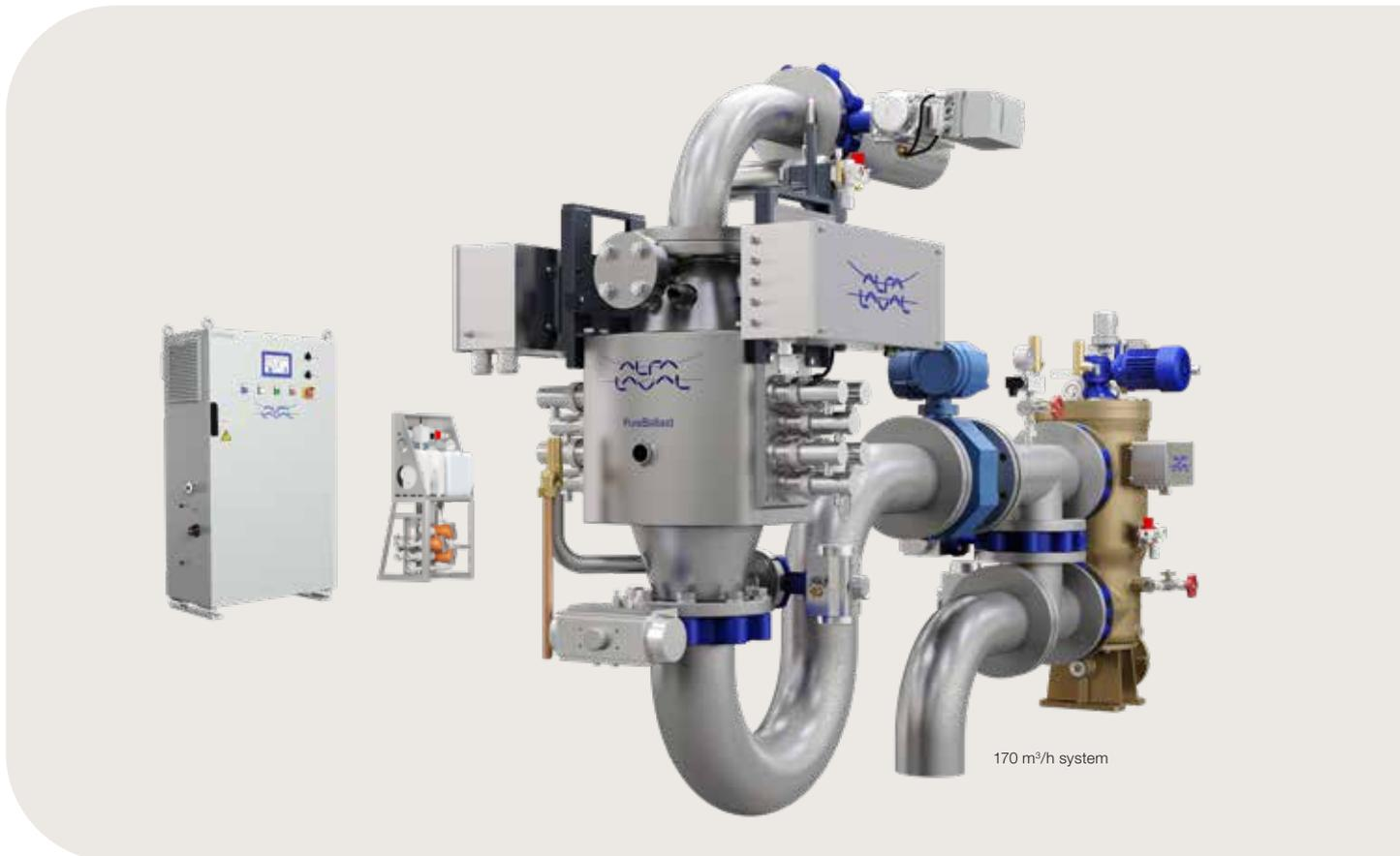
Now in its third generation, Alfa Laval PureBallast is an automated inline treatment solution for the biological disinfection of ballast water. Operating without chemicals, it combines initial filtration with an enhanced form of UV treatment to remove organisms in accordance with stipulated limits.
