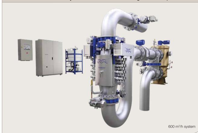
Now in its third generation, Alfa Laval PureBallast is an automated inline treatment solution for the biological disinfection of ballast water. Operating without chemicals, it combines initial filtration with an enhanced form of UV treatment to remove organisms in accordance with stipulated limits.
