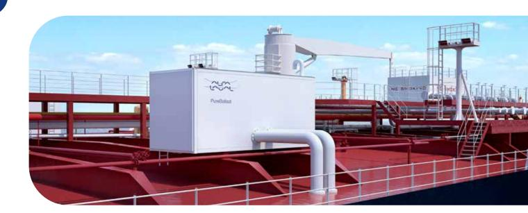
Alfa Laval has developed standard deckhouse solutions for Alfa Laval PureBallast 3 Ex ballast water treatment systems. Each deckhouse is delivered as a pre-assembled solution, including the PureBallast 3 Ex system and all internal piping and wiring, for easy integration into the vessel. If needed (see below), a booster pump unit can be integrated to ensure sufficient pressure without modifications to the existing ballast pumping system.
