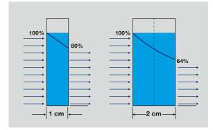
An example of UV transmittance (80%), showing the decrease in light intensity with distance from the source. Note the limited light remaining after passing through 2 cm of unclear water.
