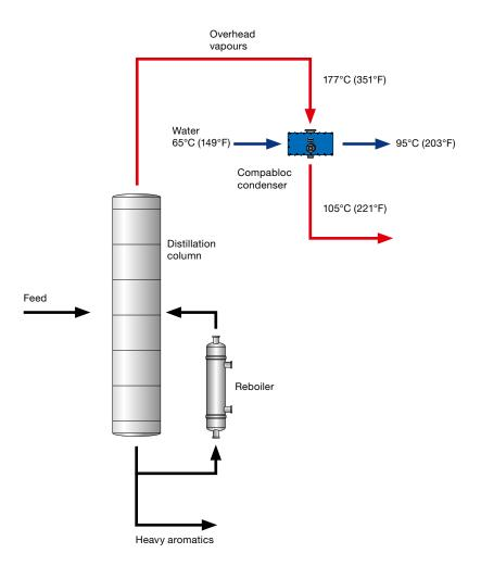
Replacing an existing air-cooled heat exchanger on top of a distillation column with an Alfa Laval Compabloc let the company save energy valued at approximately 1.25 million euros annually. Payback time, including the installation cost, was less than 6 months.
