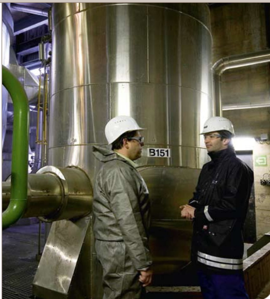
Sven Fastré of BASF and Daniel Arguelles of Alfa Laval deep in discussion in front of the flash vessel used in BASF's ammonium sulphate concentration process.
