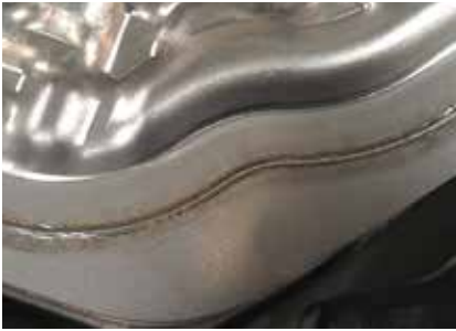
Figure 4.6 Laser welding is a much more exact technique than plasma welding and does not heat the stainless steel plates nearly as much. The result is a better and stronger joint that is less susceptible to fatigue.
