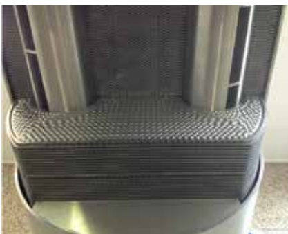
Figure 4.5 In Alfa Laval's DuroShell heat exchanger, the inlet and outlet tubes transverse the entire plate pack, adding strength where it is needed most. This design combats fatigue problems and improves the flow distribution, which in turn increases heat transfer efficiency.
