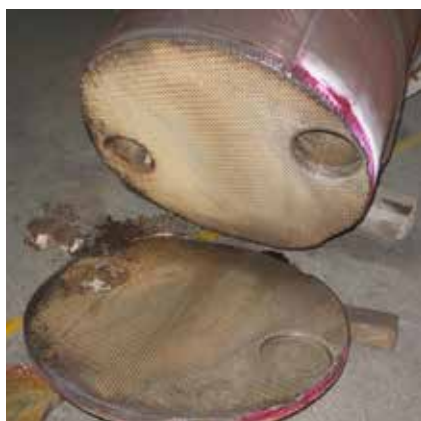
Figure 3.1 Conventional plate-and-shell heat exchangers subjected to high, varying temperatures and pressures often have problems with leakages around the port holes due to material fatigue. A few, seemingly small, design improvements can eliminate this problem.
