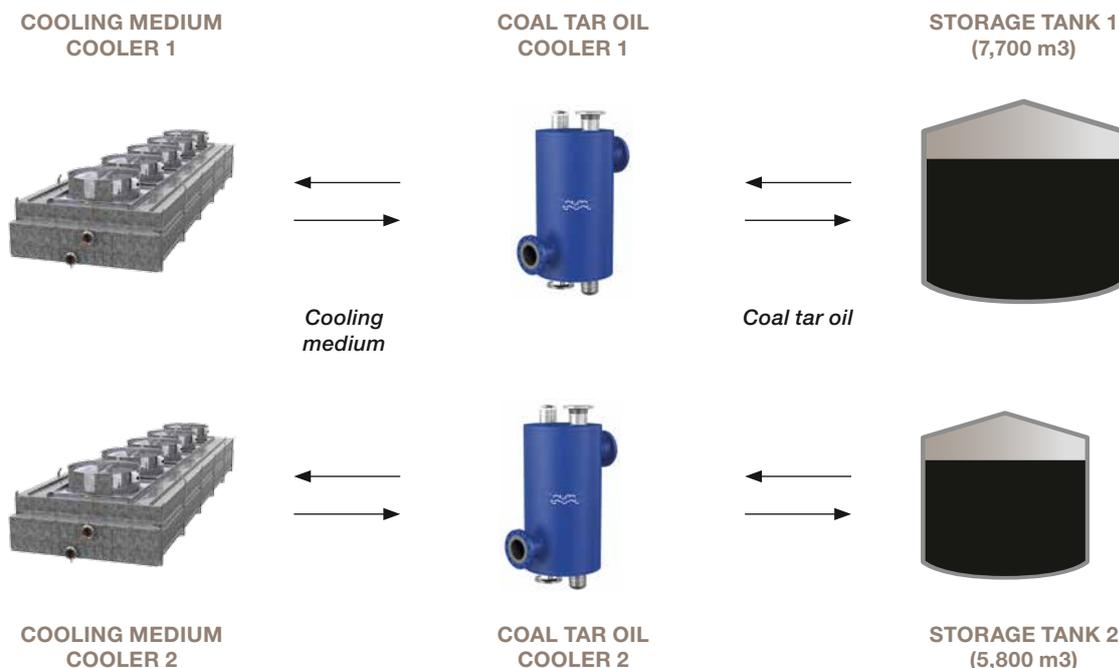
The ability to operate with crossing temperatures and the small temperature approach make DuroShell highly efficient in cooling duties. For Rütgers this means the cooling medium can be better utilized, with lower costs for piping and pumps as a result, as well as lower costs for pumping the cooling medium.
