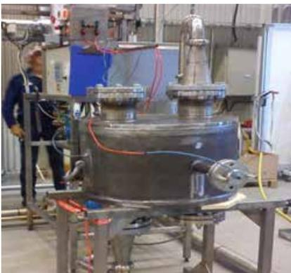
Figure 4.7 Lab tests of Alfa Laval DuroShell.
