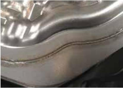
Figure 4.6 Laser welding is a much more exact technique than plasma welding and does not heat the stainless steel plates nearly as much. The result is a better and stronger joint that is less susceptible to fatigue.
