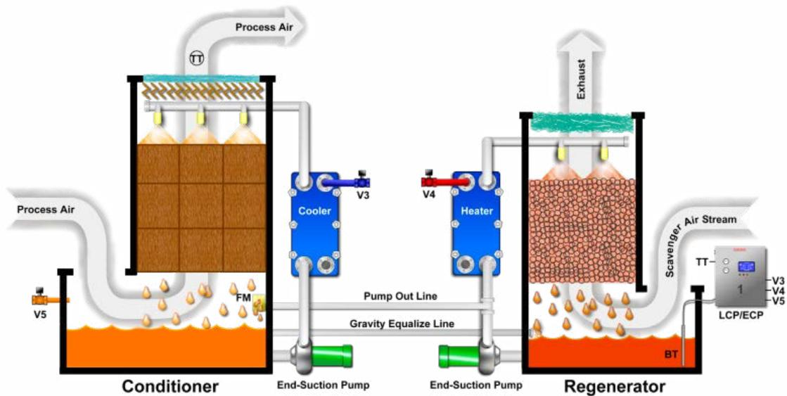
Figure 1. Liquid desiccant system schematic
