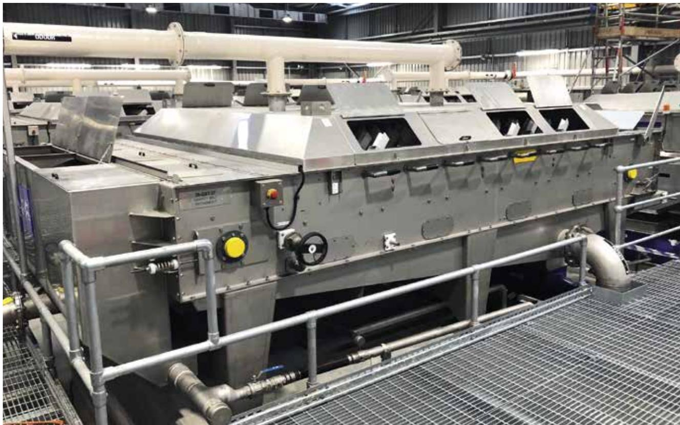
AS-H 300 Belt Thickeners processing waste activated sludge (WAS) and Three-Phase Separator (TPS) sludge.
