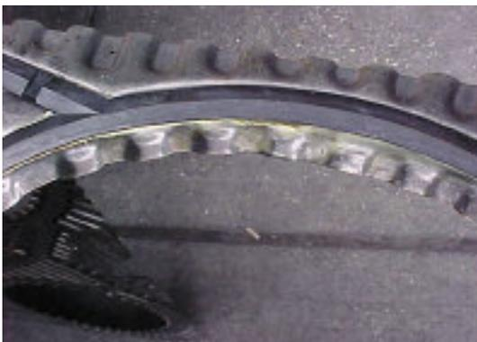
This regasketed plate suffered mechanical damage to the inner port flute due to the use of non-Alfa Laval gaskets. Therefore the plate pack will not seal properly.
