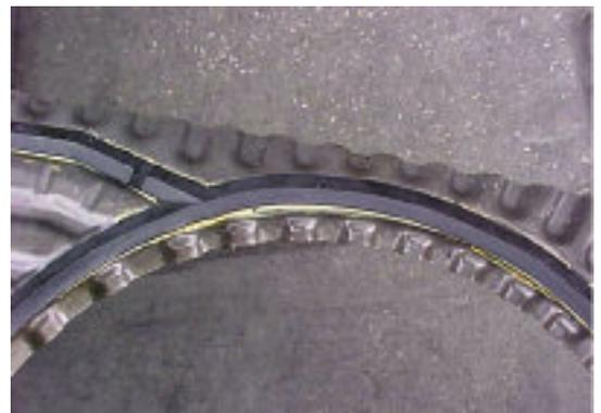
Port gasket is glued off-centre of the groove.
