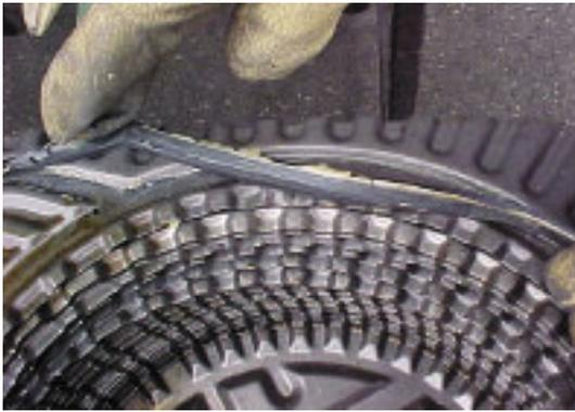
Glue has been pushed to one edge of the gasket during curing causing the gasket to sit proud with no adhesion within the gasket groove. The gasket could be lifted by finger. Sealing at this location is unlikely.
