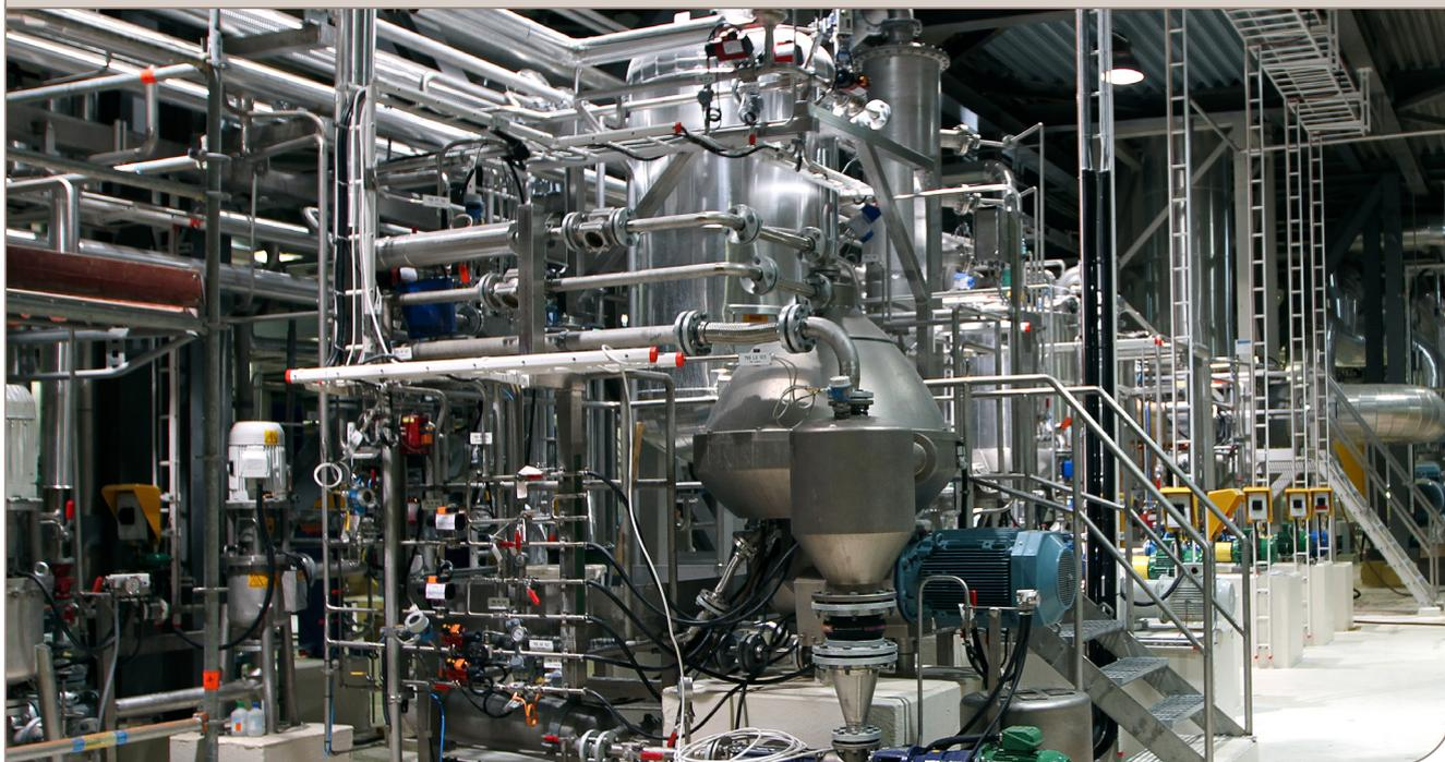
Increased yield, higher product quality and a more sustainable process were some of the improvements Swedish pulp producer Södra Cell experienced when upgrading the tall oil plant in its Värö mill to a TOPP5000 system. The new plant was supplied by HEAD Engineering and is based on Alfa Laval high-speed separators.
