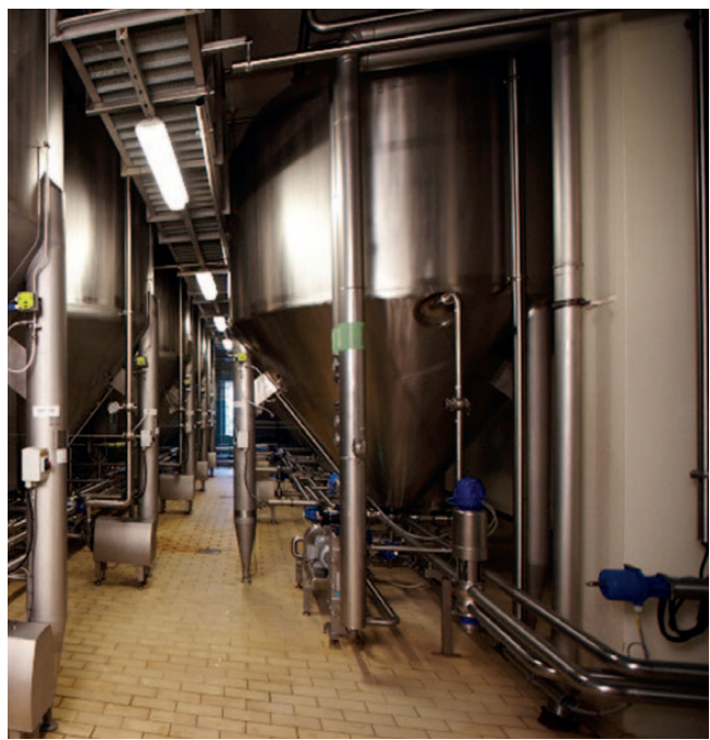
In the yeast storage tanks the Iso-Mix system ensures a homogeneous yeast slurry and improved microbiological quality.
