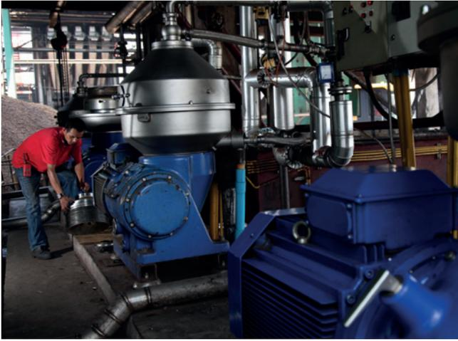
More than 10 Alfa Laval separators are used to recover crude oil, and to remove gum before the refinery's bleacher.
