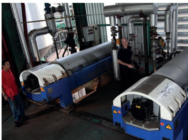
In the oil mill Alfa Laval decanters clarify and purify the crude palm oil.
