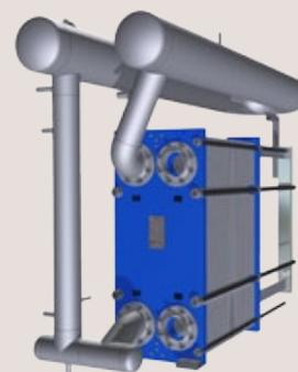
The U-Turn liquid separator is especially designed for use with plate heat exchangers in ammonia applications. It is lightweight and compact in design, making it easy to install. It can cover ammonia capacities from 200 to 1,400 kW at 0°C evaporation temperature and from 50 to 500 kW at -40°C evaporation temperature.
