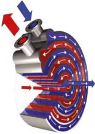
The spiral flow pattern in a spiral heat exchanger ensures a continuous, ultra-efficient self-cleaning effect.
