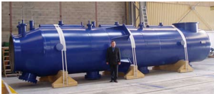
Spiral heat exchanger column supplied by Alfa Laval. The unit is 11.5 metres high and 2.1 metres in diameter.
