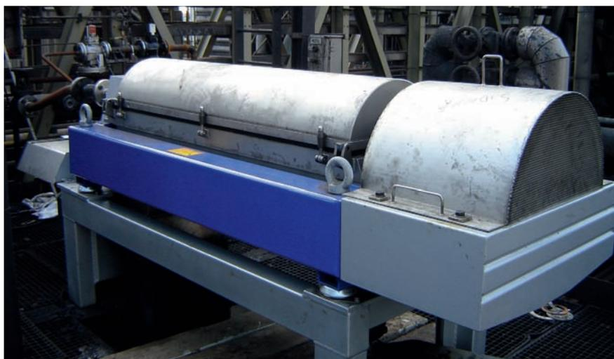
Alfa Laval CHNX 418 two-phase decanter installed at ArcelorMittal Gent for coal tar recovery.
