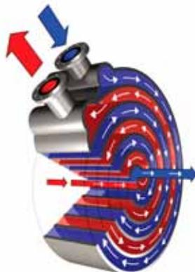
A spiral heat exchanger is circular with two concentric spiral channels, one for each fluid. The curving channels provide extremely efficient heat transfer.
