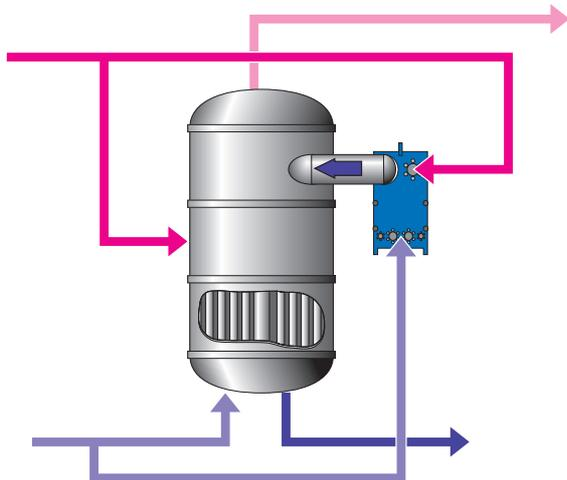
The plate evaporator installed as a booster to an existing effect
