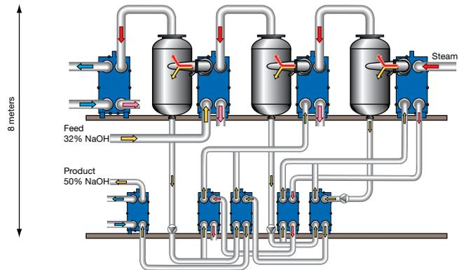
Alfa Laval's plate evaporator system is extremely compact. To the left a solution with shell-and-tubes heat exchangers and above a solution with plate heat exchangers for the same effect.
