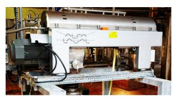
A brewery in Wales saves 5 to 7 % of wort, thanks to an Alfa Laval decanter centrifuge that recovers wort from trub in the whirlpool. In addition, the brewery can add the dry trub material from the centrifuge to the spent grains and sell it for cattle feed.
