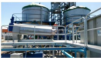
Alfa Laval Screw Press dewaters biological activated sludge, high on fats, oil and grease at a salmon processing factory at a remote island in Chile, where electricity is a scarce resource, eliminating the need – and costs - to transport wet sludge to the main land for dewatering and disposal.
