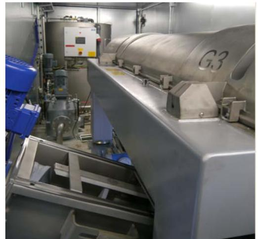
*At IFAT 2016 Alfa Laval presents a complete containerized ALDEC G3 Decanter system equipped with everything to run field tests for cost- and energy efficient thickening and dewatering of municipal and industrial sludge.*
