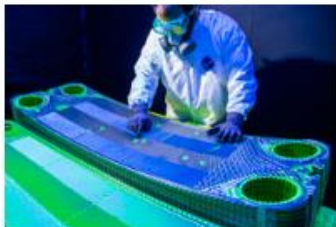
Crack and deformity detection
