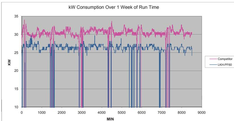
Actual kilowatt test results – with Alfa Laval's LKH-PF60 15% lower (in blue) compared to competitor's less efficient pump (in pink)
