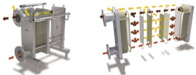
Flow pattern in a plate-and-frame unit. Red is feed/retentate. Yellow is permeate.
