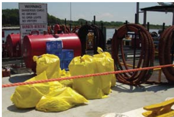
Wrapping disposable filters from filter pot in plastic bags for disposal
