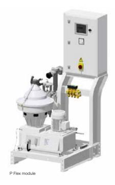
A P Flex module is a compact separator module that can be built to a customer-specified configuration from a wide range of modular skids and blocks, including any type of heater and a sludge removal kit. Multi-modules are possible, as well as mixed modules including one or more P separators for the simultaneous treatment of different types of mineral oils. All P Flex modules are factory tested to ensure faster start-up and commissioning.
