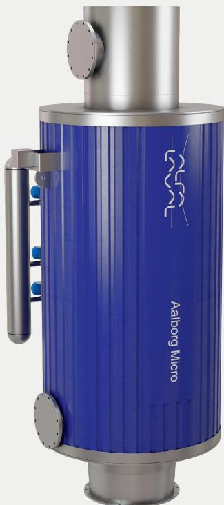
The Alfa Laval Aalborg Micro is a uniquely compact boiler/economizer designed for waste heat recovery from a vessel's auxiliary engines. Easy to install, operate and maintain, it reduces the use of the oil-fired boiler by reclaiming heat that otherwise would be lost through the exhaust gas.
