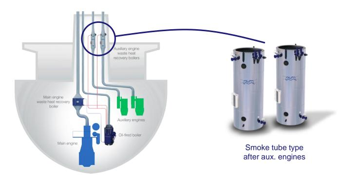
Rule of thumb – approx. 300 kg/h steam per MW Engine Power
