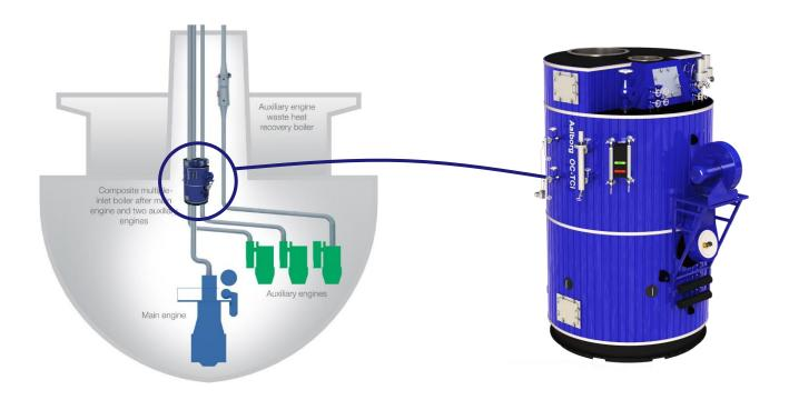
Rule of thumb – approx. 300 kg/h steam per MW Engine Power
