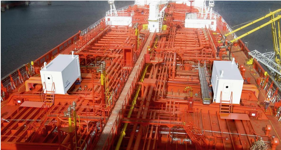
***A new Alfa Laval PureBallast 3 Ex deckhouse solution has been validated for product tankers with Framo ballast pumps. The solution allows Alfa Laval PureBallast 3 Ex to be installed on deck – without any changes to the ballast pumping system on board.***
