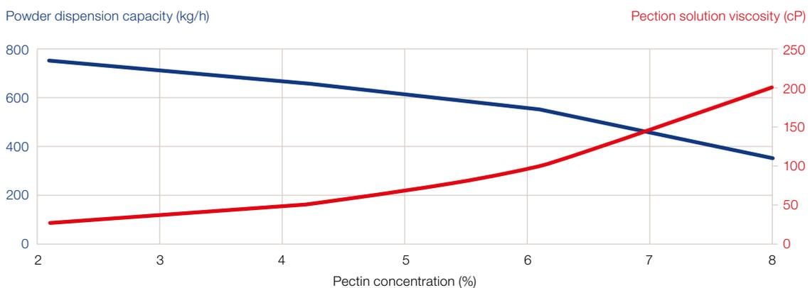
Alfa Laval Hybrid Powder Mixer: The effect of pectin concentration on dispersion capacity and pectin solution viscosity.
