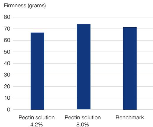
The performance of 4.2% and 8% pectin solutions used in the Alfa Laval Hybrid Powder Mixer provide the same texturing effect as that of the dry-blend pectin used as a benchmark.
