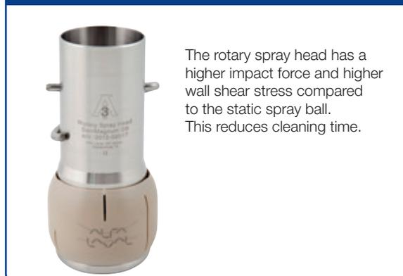
The pulsating force and impact created provide a combination of shear stress and variable falling film of cleaning fluid that covers all the internal surfaces of the tank. Compared to the static spray ball, the rotary spray head reduces the amount of cleaning time required to achieve the desired cleaning results.
