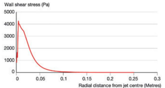
The wall shear stress in the footprint of an impinging jet from a rotary jet head, with water temperature at 20°C and pressure at 5 bar, is shown.
