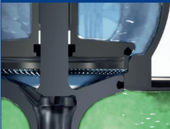
**Seat lift:** The upper valve plug is raised off the seat thus cleaning plug seal, seat and leakage chamber through CIP flow.
