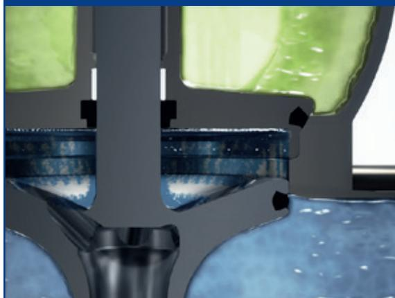
**Seat push:** The lower plug is pushed downwards thus cleaning the plug seal, seat and leakage chamber through CIP flow.
