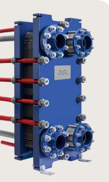
Semi-welded technologies combine the flexibility and serviceability of standard gasketed plate heat exchangers, while enabling reliable operation at higher design pressures. Modern designs with optimized sealing further reinforce the heat exchanger's dependability. Semi-welded plate heat exchangers can also offer high resistance against ice formation and fatigue stresses from pressure and/or temperature variations.
