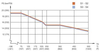
Min temperature -50  $^{\circ}\text{C}$  (-58  $^{\circ}\text{F}) with connection tubes made of carbon steel.$
