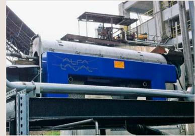
**Pulp mills across the world**, for example in Turkey, Russia and Chile, have installed decanter centrifuges for green liquor dregs dewatering. The new equipment brings many benefits:
