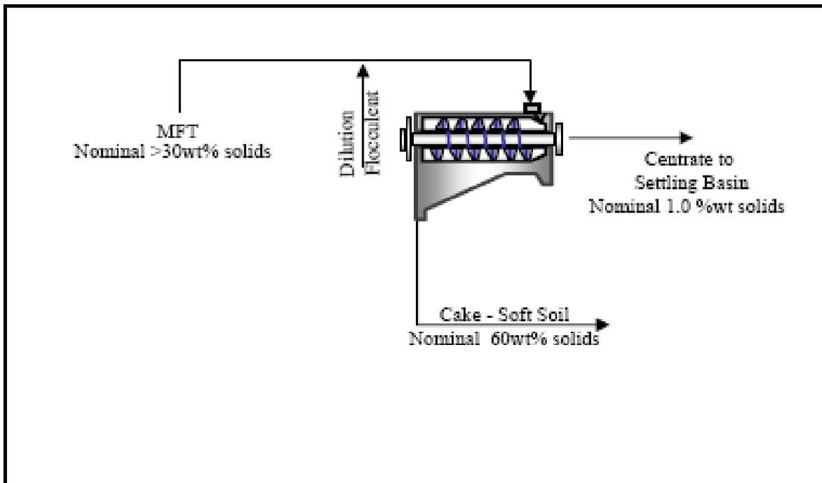
Figure 7. The decanter in the process
