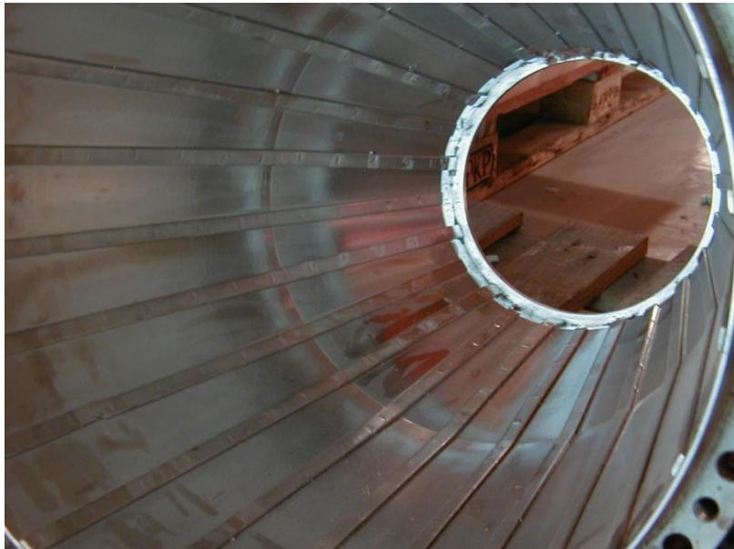
*Figure 5. Ribs in the centrifuge bowl*
