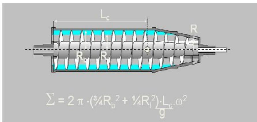
Figure 3. Sigma factor & centrifuge performance
