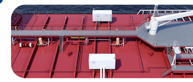
The technical teams for Alfa Laval ballast water treatment systems and Framo pumping systems have developed a solution for providing additional pumping head when PureBallast 3 Ex is installed in a deckhouse. By ensuring that the PureBallast 3 Ex system can handle its own pressure requirements, the optional booster pump unit (BPU) removes the need for changes in the existing ballast pumping system, thereby retaining its optimization and the vessel's cargo offloading rates.
