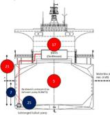
Since the ballast water treatment system requires around 17 mlc, the installed ballast pumps alone will not support proper backflushing, which may result in failure and the shutdown of cargo operations. Installing a BPU in the deckhouse will remove this problem by ensuring adequate discharge head in the ballast water treatment system.
