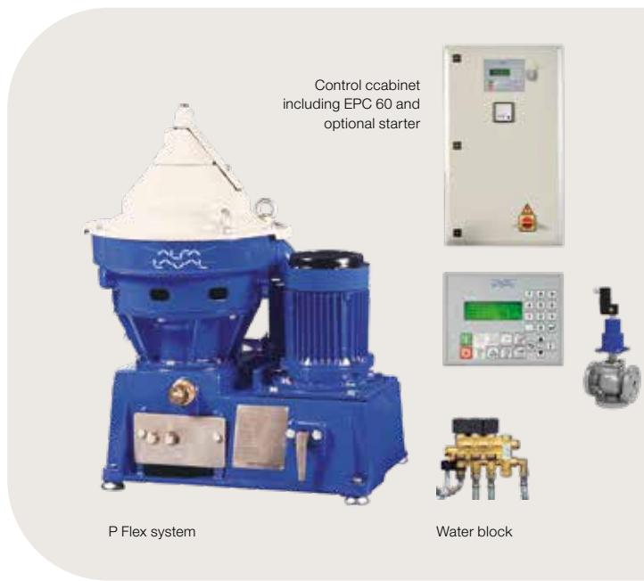
A P Flex module is a compact separator module that can be built to a customer-specified configuration from a wide range of modular skids and blocks, including any type of heater and a sludge removal kit. Multi-modules are possible, as well as mixed modules including one or more P separators for the simultaneous treatment of different types of mineral oils. All P Flex modules are factory tested to ensure faster start-up and commissioning.
