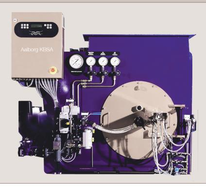
The Aalborg KBSA steam atomising burner is designed for use on our side-fired boilers and can be delivered premounted. The use of oil flowmeter and modulation of the atomizing steam pressure ensures a stable combustion at all loads, also in the lower end. All burner mountings are arranged to ensure easy installation and maintenance.
